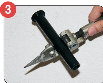
3 Cut tube to length using pipe cuner or hacksaw.
