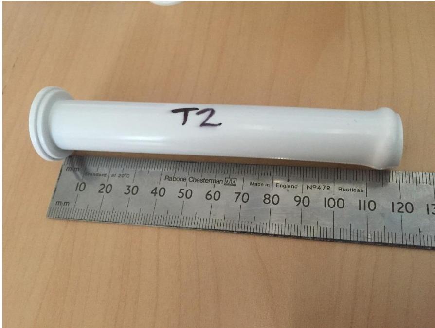
Figure 5 – Compression loads of circa 595 Kg with only minor deformation.
